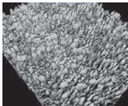
Figure 6 - Sequence of filters in which undulations and forms are removed. Nanotite with Gaussian filter of 50 \times 50 \mu\text{m} .
