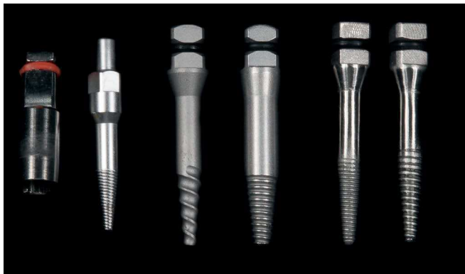
Figure 16 - Tapered removers available in the dental market of the brands: Nobel Biocare (Zurich, Switzerland), Kopp (Curitiba, Brazil) and Maximus (Contagem, Brazil), from left to right, respectively.
