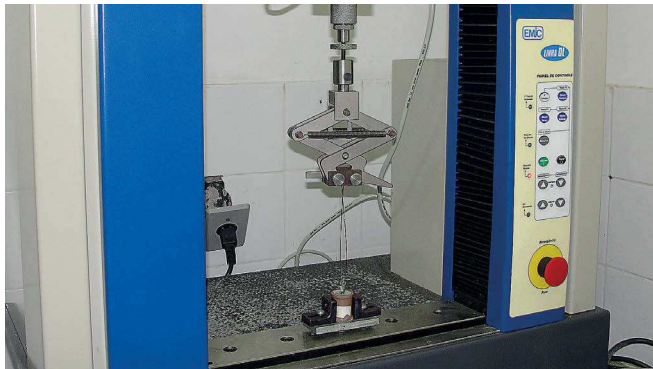
Figure 9 - EMIC machine with the specimen positioned for testing.
