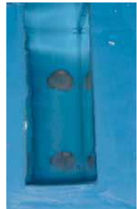
FIGURE 5 - After epoxy resin manipulation, it was poured carefully to avoid incorporation of air bubbles.
