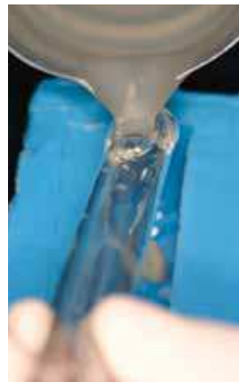
FIGURE 5 - After epoxy resin manipulation, it was poured carefully to avoid incorporation of air bubbles.
