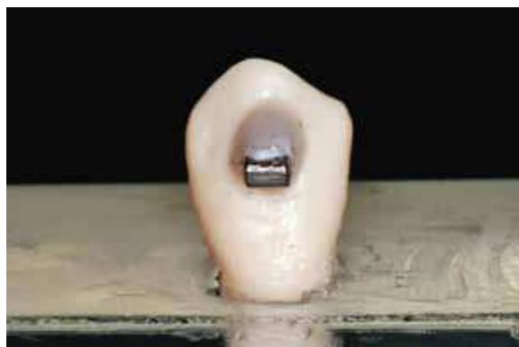
FIGURE 7 - Photoelastic model with 'crossed' tubes in position.
