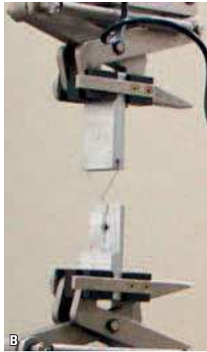
FIGURE 3 - U-shaped stainless steel 0.021x0.025-in wire device used for bonding the brackets.
