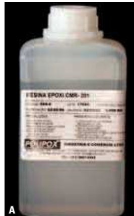
FIGURE 5 - Photoelastic resin: A) COMPONENT "A" EPOXY resin, flexible CMR-201 and B) Component "B" Flexible CME-252 Hardener
