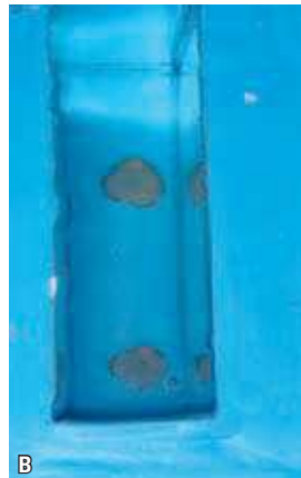
FIGURE 4 - After placement of teeth in their respective places, resin with photoelastic properties was manipulated and inserted in negative mold to obtain photoelastic model.
