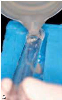
FIGURE 4 - After placement of teeth in their respective places, resin with photoelastic properties was manipulated and inserted in negative mold to obtain photoelastic model.
