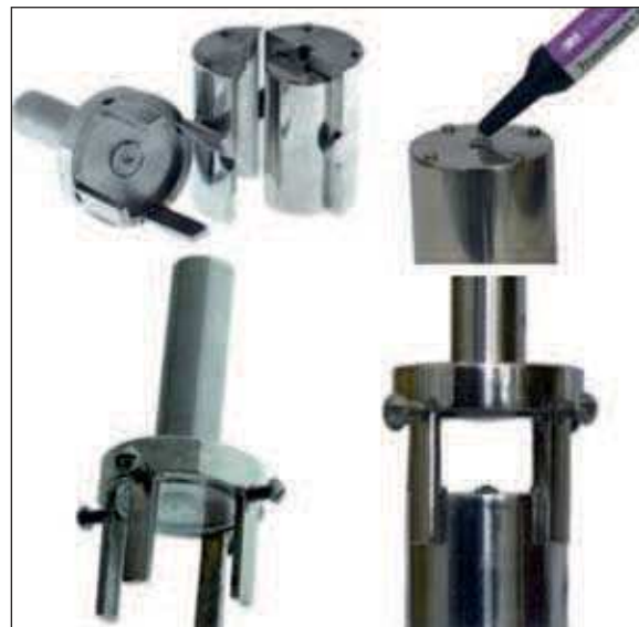
FIGURE 2 - Bonding device used to ensure standardization. Illustration of how the brackets were bonded to the acrylic resin discs.
