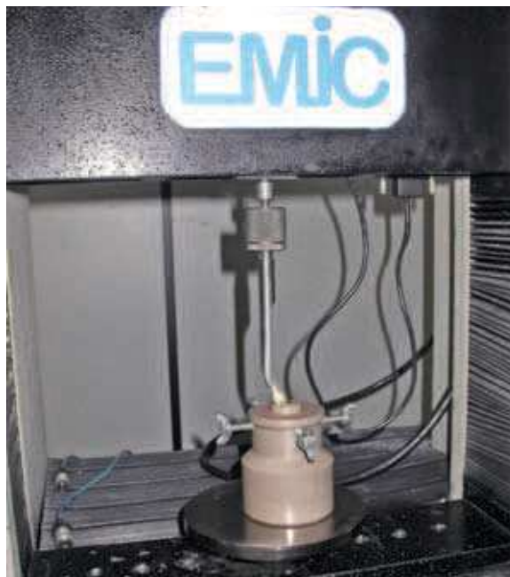
FIGURE 1 - Device fabricated to maintain the specimen stable during the test.
