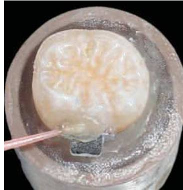
FIGURE 3 - Applying resin to occlusal surfaces of tube/tooth interface with aid of brush dipped in adhesive.
