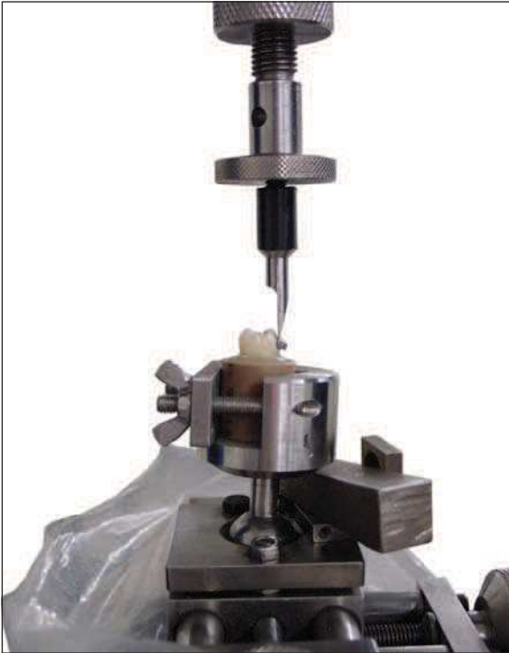
FIGURE 6 - Position of the shear bond strength testing device.
