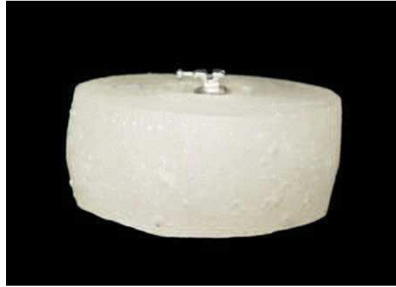
FIGURE 5 - Specimen bonded to ceramic veneer attached to acrylic resin cylinder with bracket base parallel to cylinder surface (lateral distal view of bracket).
