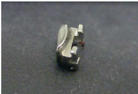
FIGURE 3 - Gemini bracket bases filled with resin for subsequent bonding to surface of metal cylinders. Observe the flattening of the bases accomplished with Transbond XT light cure resin. This procedure was used prior to bonding all brackets under test.
