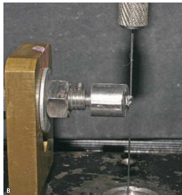
FIGURE 2 - A) Front view of self-ligating bracket bonded to metal cylinder with compensatory angulation to ensure traction is performed with no pre-angulation or torque. Total absence of angulation (tip) can be confirmed by the vertical alignment of the markings on the metal cylinder and copper colored part seen in the background. B) Side view of the same bracket described during traction of stainless steel 0.019 x 0.025-in cross-section wire.
