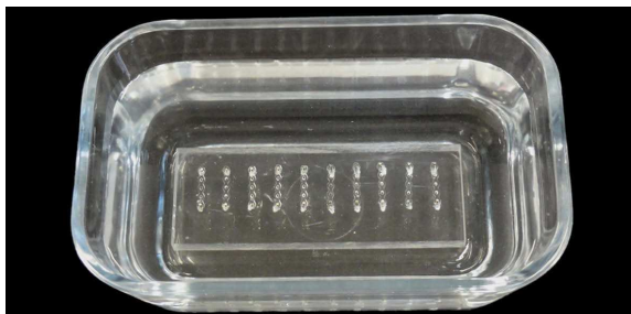
FIGURE 4 - Acrylic resin plate immersed in artificial saliva.
