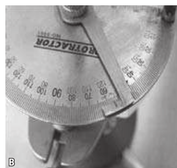
FIGURE 8 - Model positioned with the hand over the cusp of the right maxillary canine (A); protractor pointing the position of the right maxillary canine at 33.5° (B).
