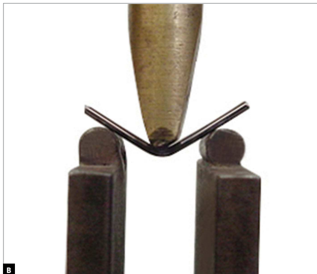
Figure 1 - In vitro evaluation of flexural strength of different brands of screw expanders. (A) The screw stem positioned before the test, (B) after flexural test.
