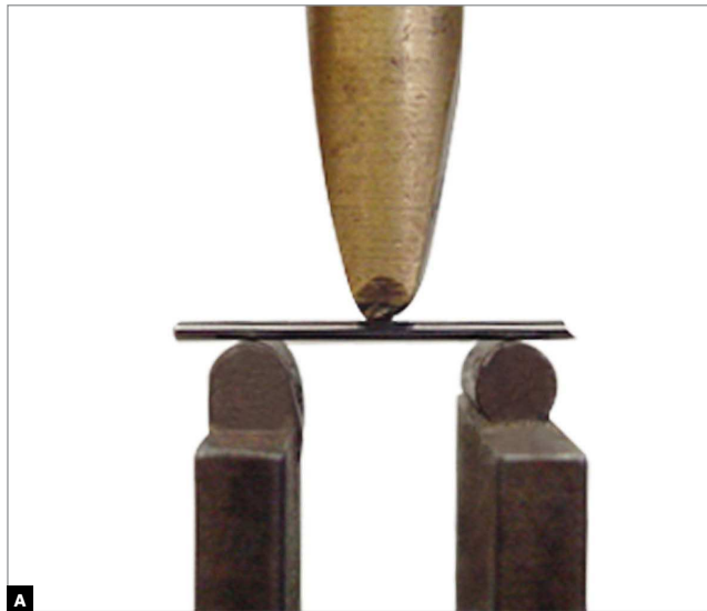
Figure 3 - Stress x deformation showing the flexural strength of the Forestadent screw.
