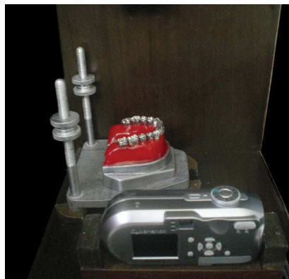
Figure 5 - Wooden device to standardize the registration of the phases (initial, 0.014-in, 0.016-in, 0.018-in and 0.020-in) by means of digital photographs in the orthogonal norm to the sagittal plane.
