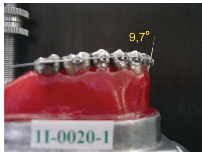
Figure 6 - Sequence of photographs to obtain lower incisor tipping at all stages (initial, 0.014-in, 0.016-in, 0.018-in and 0.020-in).
