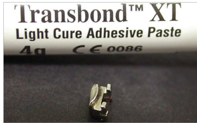
Figure 3 - Gemini bracket bases filled with resin for subsequent bonding to the surface of metal cylinders. Note how the bases were levelled (filled) with Transbond XT light cure adhesive.
