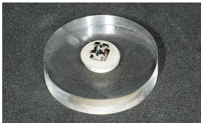
Figure 3 - Orthodontic Brackets bonded with Transbond XT light-cured resin onto previously treated surfaces.
