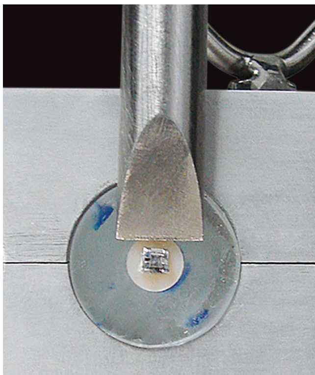
Figure 4 - Bracket shearing in an Emic DL 10000 MF universal testing machine. Note the metallic support for fixation of specimens.
