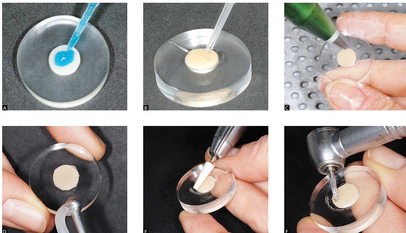
Figure 2 - Surface treatment using: A) 37% phosphoric acid, B) hydrofluoric acid, C) aluminum oxide blasting, D) sodium bicarbonate blasting, E) mounted stone, and F) diamond bur.
