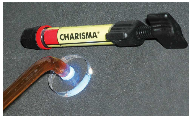
Figure 1 - Light curing of specimens filled with resin composite.
