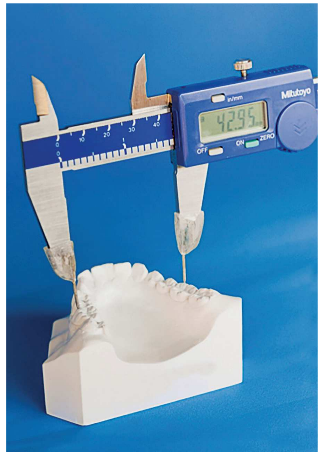
Figure 4 - Intermolar width measured on a dental cast by means of a digital caliper.
