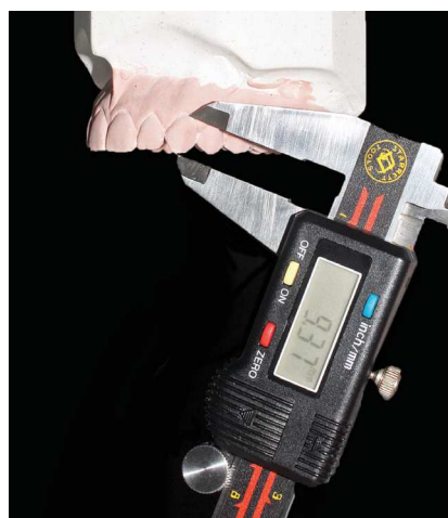
Figure 1 - Measurement of the height of the dental crown in the plaster model, with a digital caliper.
