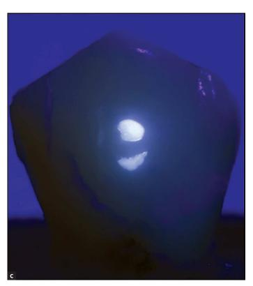
Figure 1 - A) Mannequin with bonded specimens, B) Mannequin head with bonded specimens, for composite removal. C) Specimen exposed to ultraviolet light used to measure the area of adhesive remnant (Source: Ribeiro et al.<sup>2</sup> 2017).
