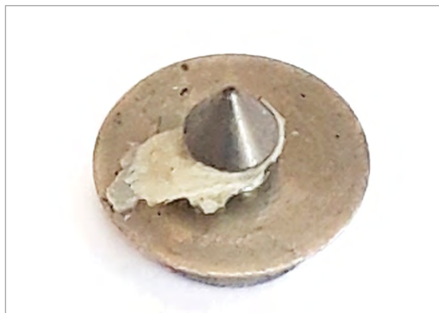
Figure 5 - Mini-implant with cohesive in bone fracture.
