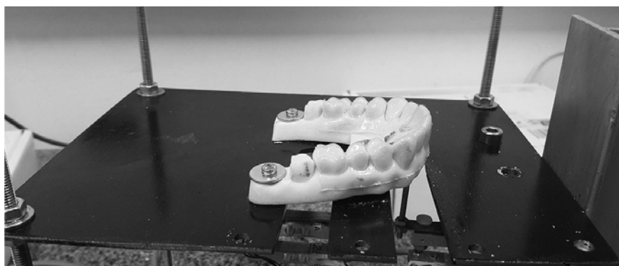
Figure 3 - 3D-printed model, with thermoplastic aligner fixed in the frame.
