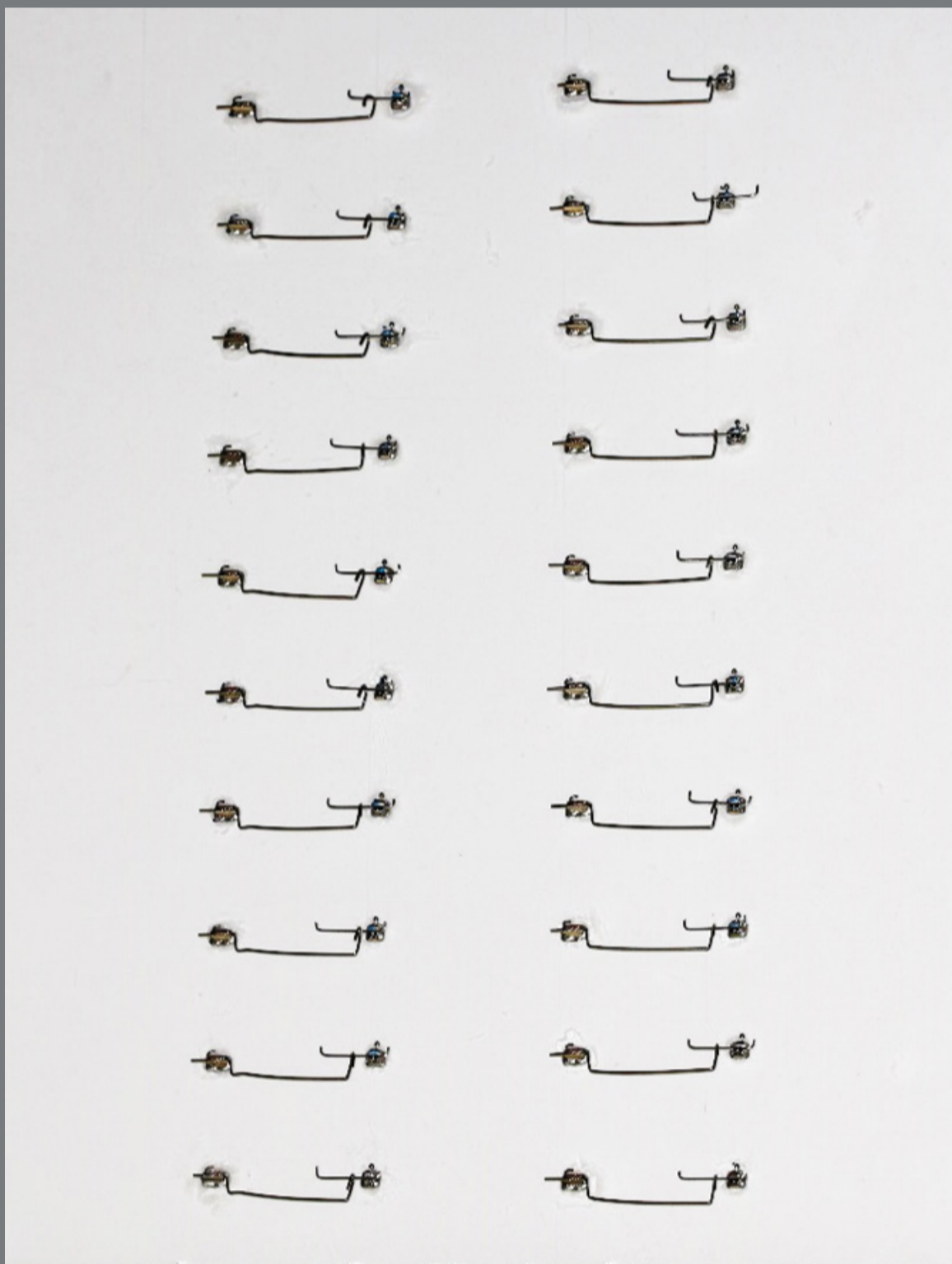
Figure 3: Custom made device, simulating the clinical activation of cantilevers, in order to keep the cantilevers activated.
