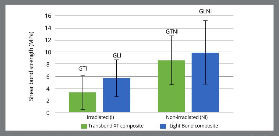
**Figure 2:** Column diagram of the average bond strength values of ceramic brackets bonded with different composite resins on enamel submitted or not to ionizing radiation. GTI = Group Transbond irradiated; GLI = Group Light Bond irradiated; GTNI = Group Transbond non-irradiated; GLNI = Group Light Bond non-irradiated.
