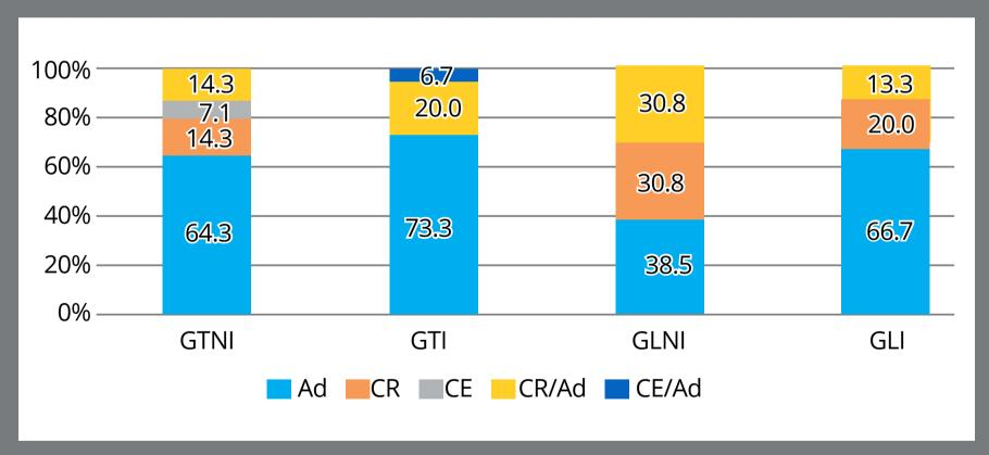
**Figure 3:** Mean fracture patterns, percentage, after shear test. Ad = Adhesive fracture; CR= Resin cohesive fracture; CE = Enamel cohesive fracture; CR/Ad = Resin/adhesive cohesive mixed fracture; CE/Ad = Enamel/adhesive cohesive mixed fracture. GTI = Group Transbond irradiated; GLI = Group Light Bond irradiated; GTNI = Group Transbond non-irradiated; GLNI = Group Light Bond non-irradiated.
