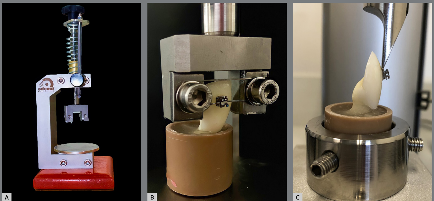
Figure 1: A) Parallelometer device. B) Sample included in the PVC cylinder with the aid of the parallelometer. C) Cylinder containing tooth fixed in a universal mechanical testing machine for shear bond strength testing.
