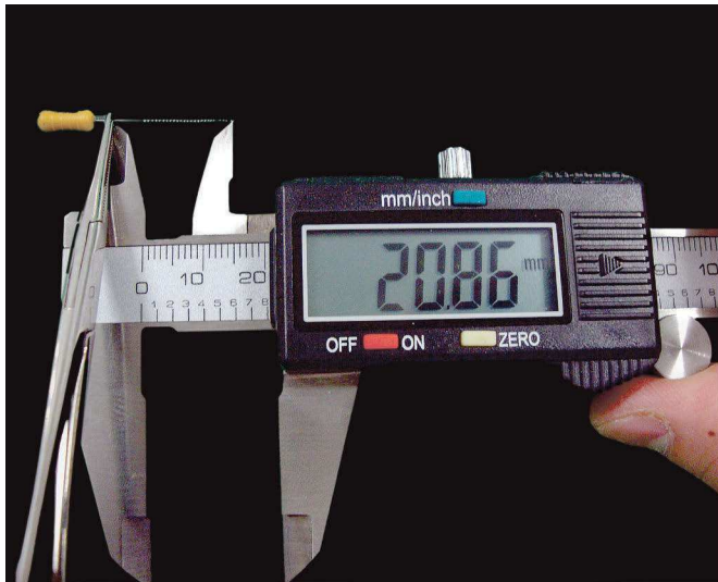
Figure 3. K-type file removed from inside the root canal and measured using a digital caliper.
