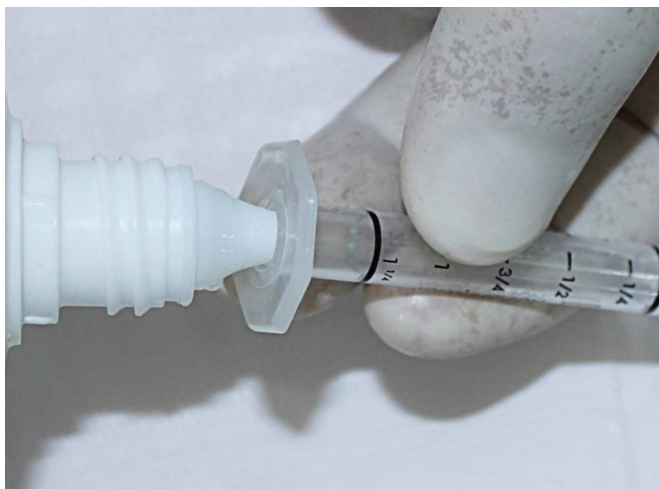
Figure 2. Syringe and Capillary Tip lubrication with propylene glycol.
