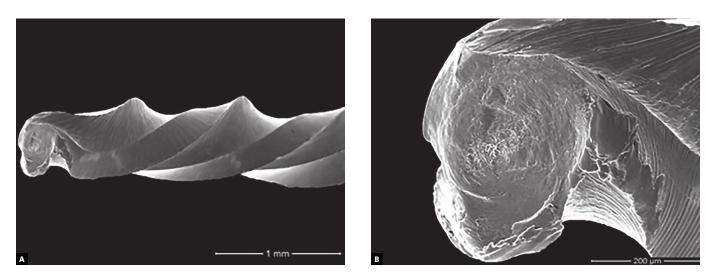
Figure 10. A) Helical shaft plastic deformation - WaveOne Large file (100x magnification). B) Fracture surface and spiral reversion at fracture site (500x magnification).
