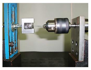
Figure 3. Photo of assembly used to apply torsional loads.
