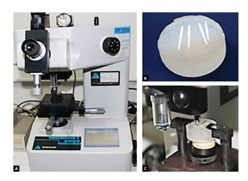
Figure 4. Micromet 2003 microindentation hardness tester (A) specimen embedded in resin plate (B); specimen positioning (C).
