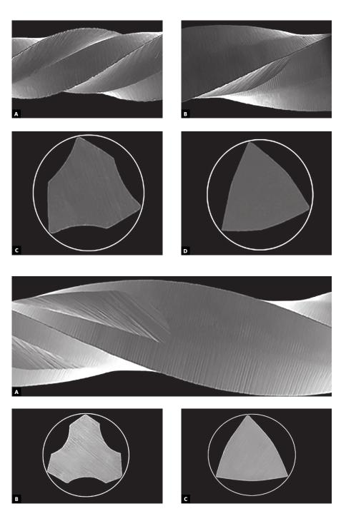
Figure 8. WaveOne Large file. Helical cutting shaft (A, B). Cross section of helical cutting shaft (100x magnification) (C, D).
