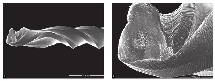
Figure 11. A) Helical shaft plastic deformation - ProTaper F4 file (100x magnification). B) Fracture surface and spiral reversion at fracture site (500x magnification).
