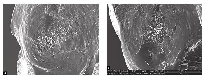
Figure 12. Ductile fracture surface: A) WaveOne Large; B) ProTaper F4 file (1000x magnification).
