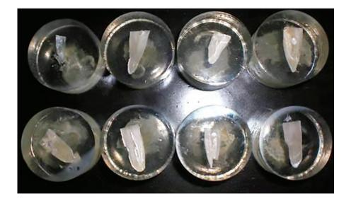
Figure 2. Samples in acrylic resin.
