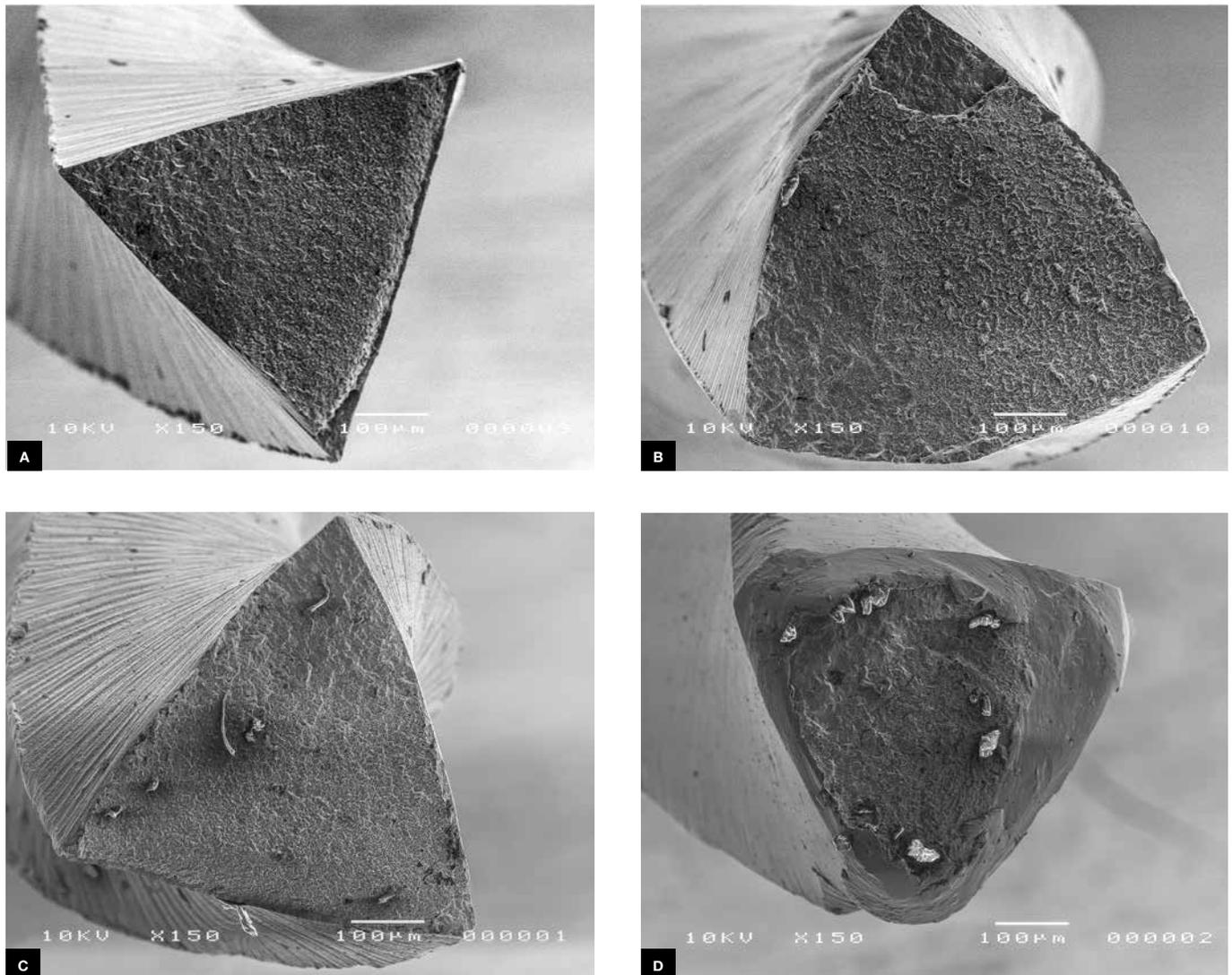
**Figure 2.** SEM images of fractured surfaces of separated fragments of (A) Hyflex CM, (B) Vortex Blue, (C) Sequence Rotary File and (D) EdgeSequel after cyclic fatigue testing. The images show numerous dimples, a feature of ductile fracture.
