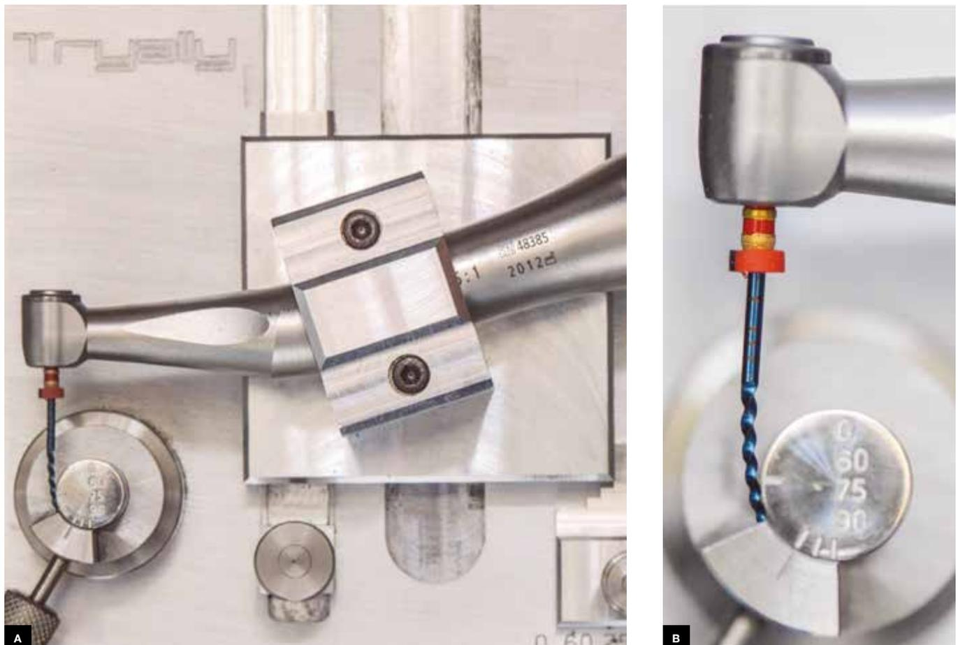
**Figure 1. A)** The instrument positioned in the cyclic fatigue test device. **(B)** The artificial canal with an angle of curvature of 60° and a radius of 5 mm.
