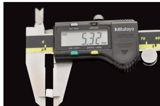
Figure 3: Measurement with a digital pachymeter of 0.01 mm precision.
