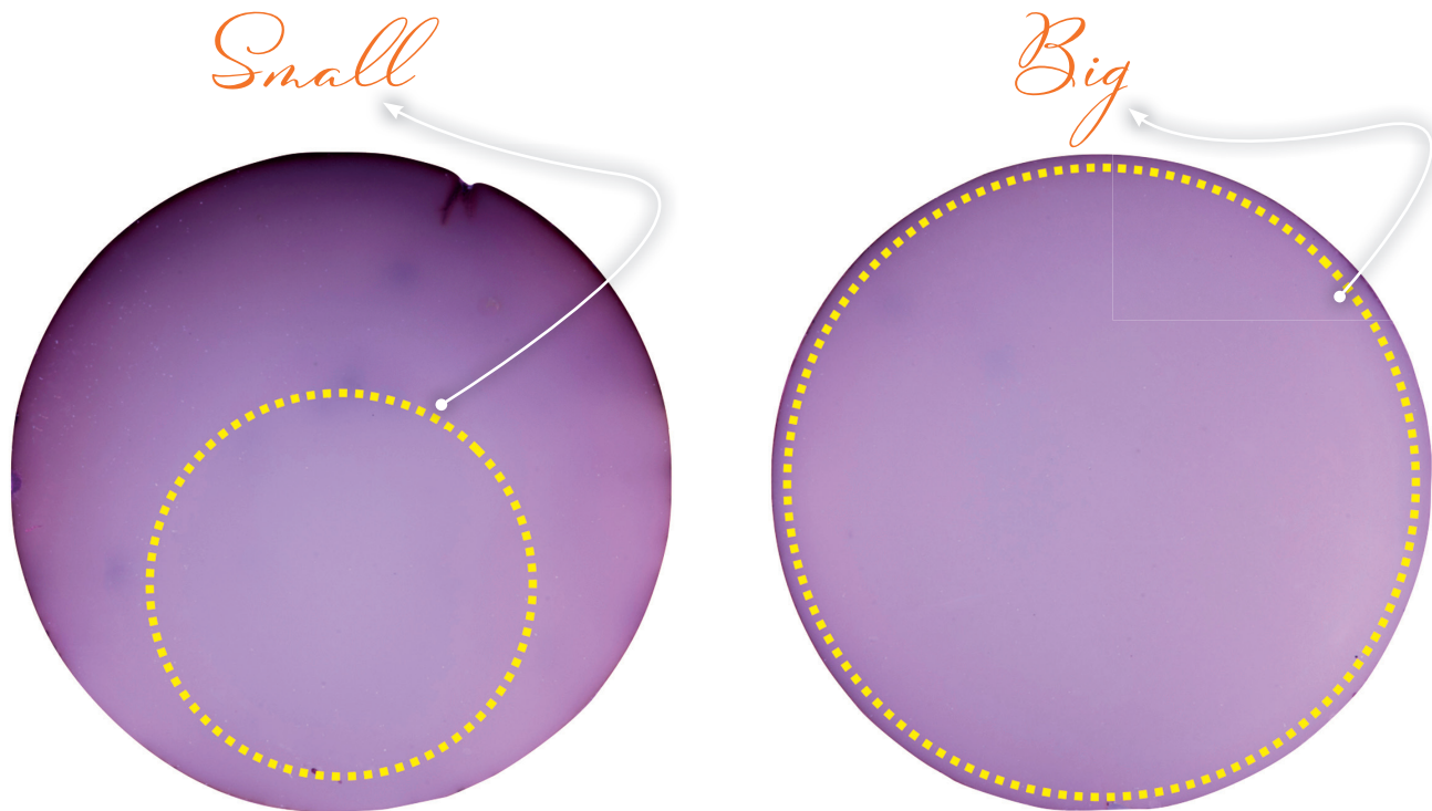
Figure 2: Resin-based composite discs with a 12-mm diameter light cured for 20 seconds using an equipment with narrow tip (left) and an equipment with tip compatible with the disc size (right). Discs were immersed in red wine for 7 days to evidence the accelerated staining of regions not covered by the light emitted by the light curing units. Yellow dashed circles represent the size of the light curing units' tips.
